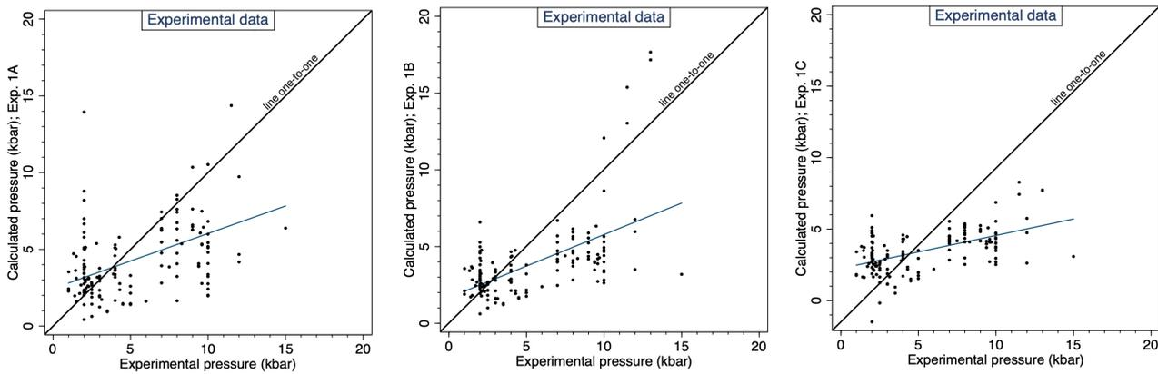
**Figure 2.** Calculated versus experimental pressures. Pressures estimated with the amphibole-only expressions 1A, 1B and 1C by Ridolfi and Renzulli [5]. Data compiled from the literature by Molina et al. [9].
