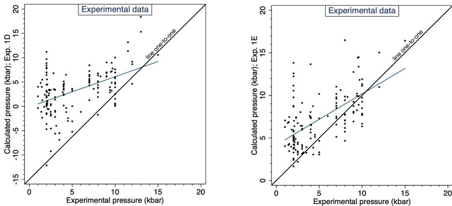
**Figure 3.** Calculated versus experimental pressures. Pressures estimated with the amphibole-only expressions 1D and 1E by Ridolfi and Renzulli [5]. Data compiled from the literature by Molina et al. [9].
