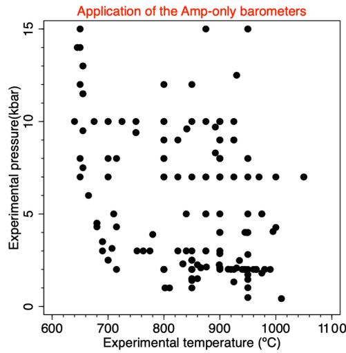
**Figure 1.** Experimental runs with amphibole having  $Mg/(Mg+Fe^{2+}) > 0.5$ . Data compiled from the literature by Molina et al. [9].
