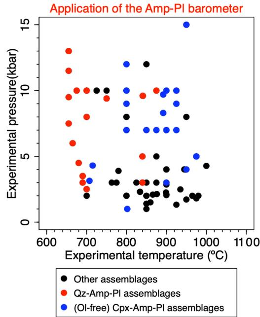
**Figure 4.** Experimental runs with amphibole having (apfu, 23O): total Al > 1, Ti: 0.05-0.27 and Fe<sup>3+</sup><1.07. Data compiled from the literature by Molina et al. [9].
