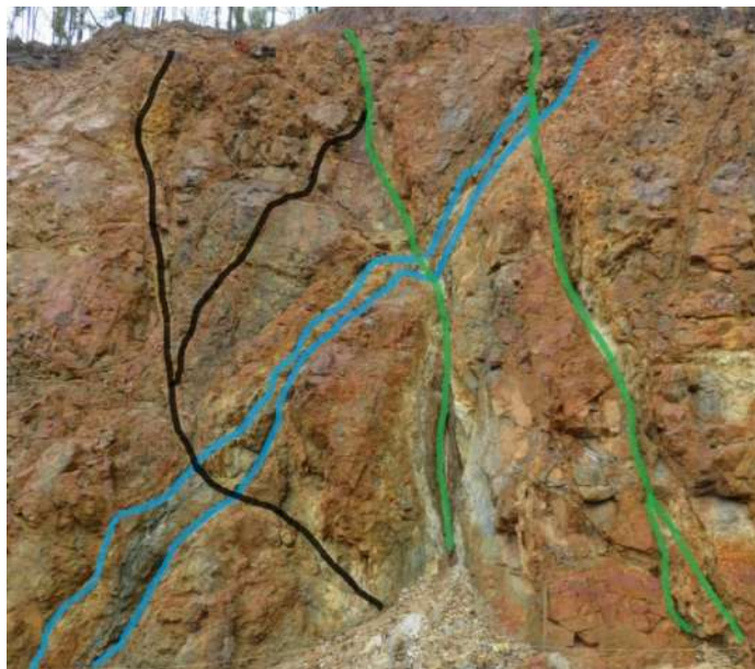
Figure 3. Major conjugate shear and vein structures in the south wall of the Strauss open-cut. All are intensely altered and mineralized. S1 – blue, S2 – green, conjugate vein - black
