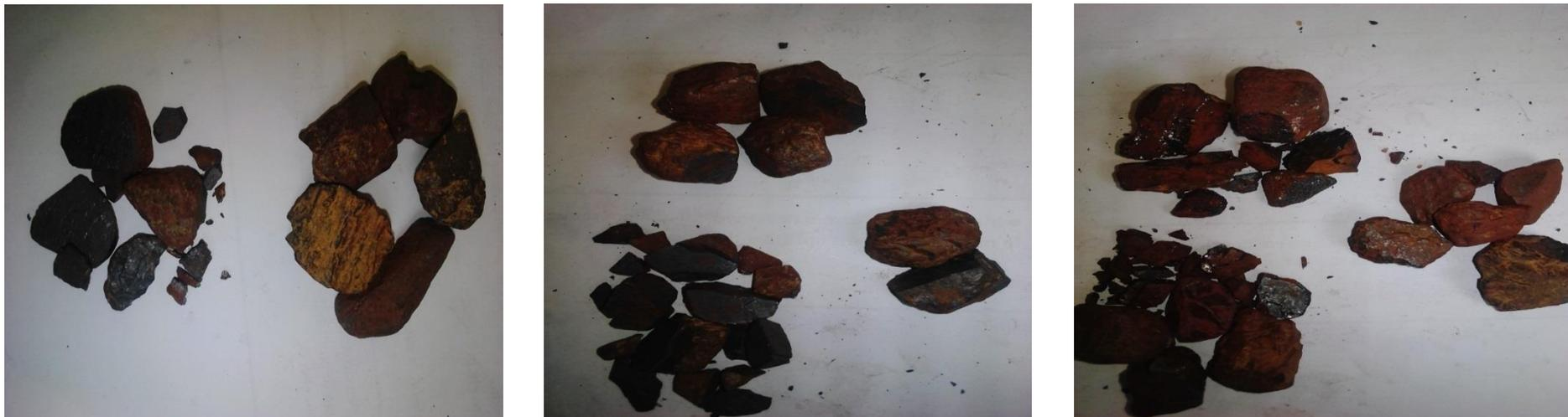
**Fig. 5.2:** Effect of structural changes on reduction behavior at different temperatures in charcoal at reduction time of 40mins. (a) 570°C (b) 700°C (c) 900°C
