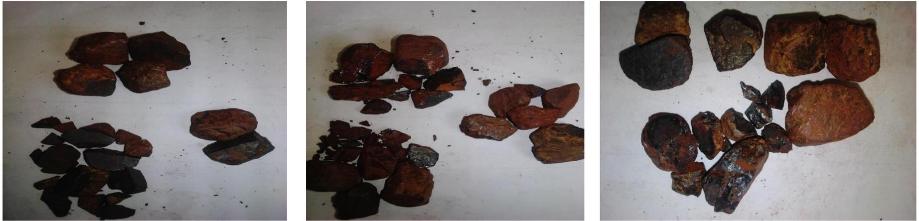
**Fig. 5.1:** Crack formation and iron grain disintegration of fired hematite ore samples of different sizes as reduced for 40mins (a) 700°C (b) 800°C (c) 1000°C
