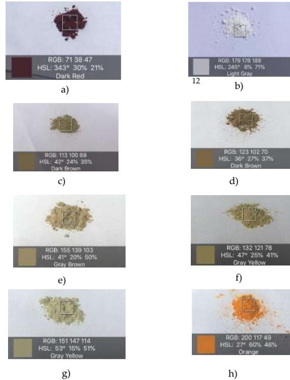
**Figure 3.** Color evaluation of samples a) Bixin; b) Montmorillonite; c) Ca-Mt-Bx; d) Fe-Mt-Bx; e) Cu-Mt-Bx; f) Mg-Mt-Bx; g) Na-Mt-Bx and h) Al-Mt-Bx.
