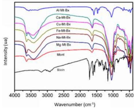
**Figure 2.** Infrared spectra for samples Na-Mt-Bx, Mg-Mt-Bx, Fe-Mt-Bx, Cu-Mt-Bx, Ca-Mt-Bx, Al-Mt-Bx, Montmorillonite and Bixina.
