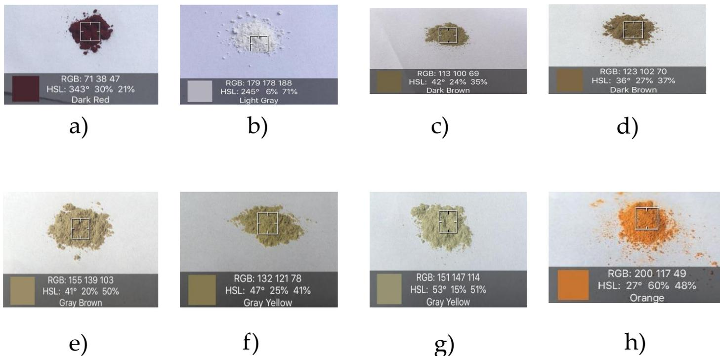
**Figure 3.** Color evaluation of samples a) Bixin; b) Montmorillonite; c) Ca-Mt-Bx; d) Fe-Mt-Bx; e) Cu-Mt-Bx; f) Mg-Mt-Bx; g) Na-Mt-Bx and h) Al-Mt-Bx.
