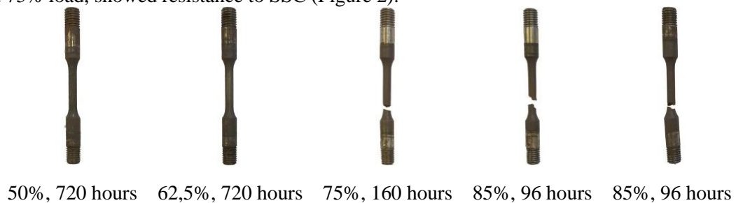
Figure 2. Samples after SSC testing
