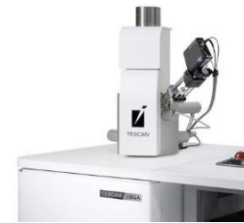
Electron Microscope Tescan VEGA 3 equipped with Inca X-Max EDS analyzer
