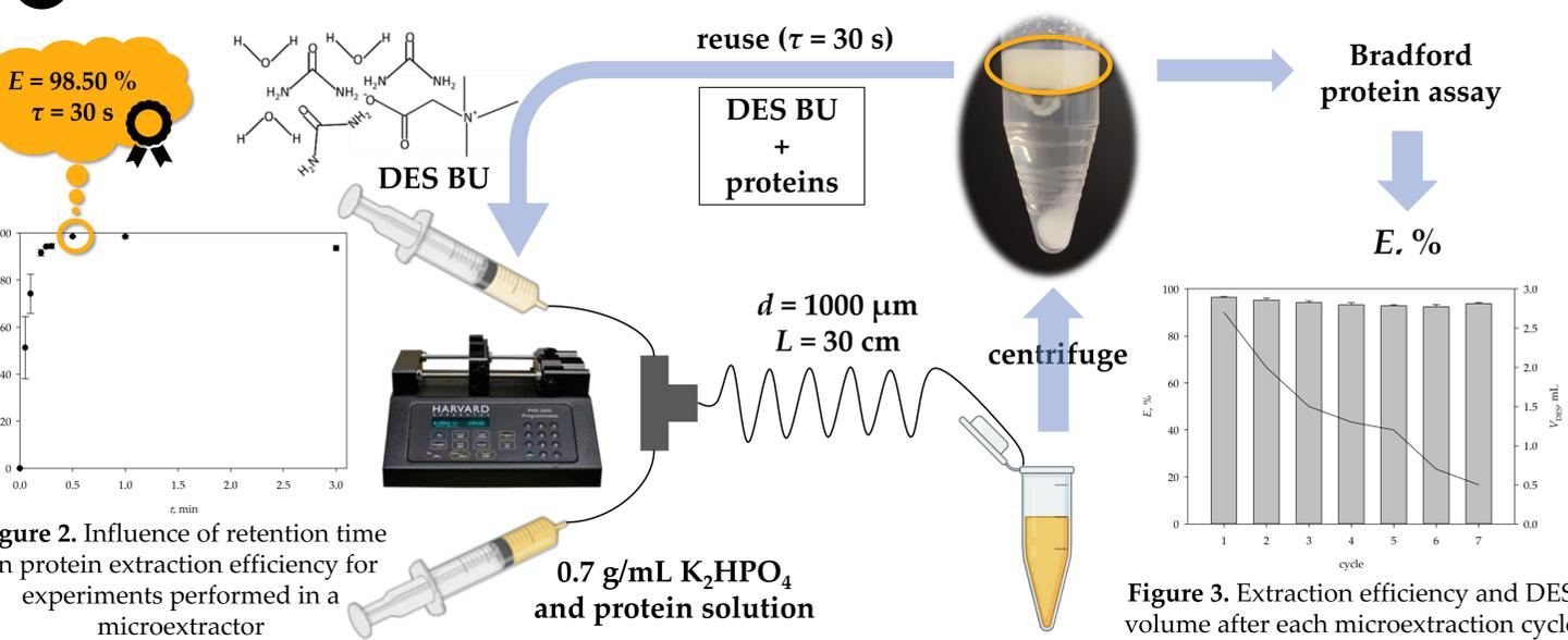
Figure 2. Influence of retention time on protein extraction efficiency for experiments performed in a microextractor
