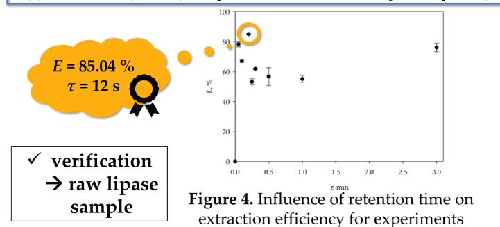
Figure 4. Influence of retention time on extraction efficiency for experiments performed with raw lipase in a microextractor
