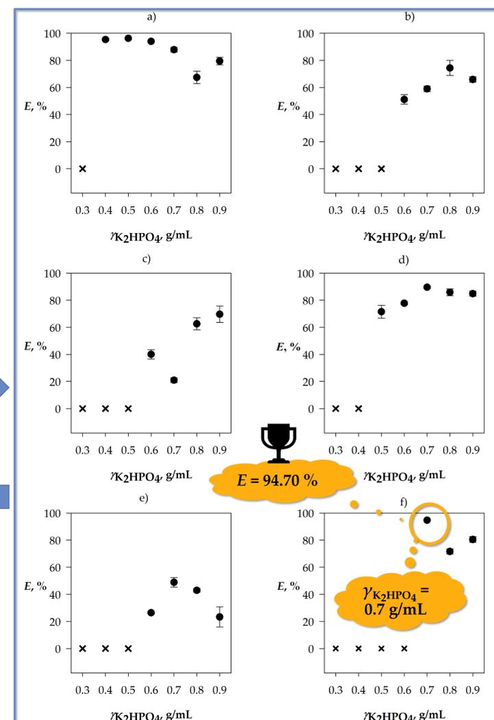
Figure 1. Influence of  $K_2HPO_4$  concentration on protein extraction efficiency in ATPS based on (a) ChU, (b) BGly, (c) ChGly, (d) ChGlc, (e) ChEG and (f) BU (x no phase formation, • two-phase system)
