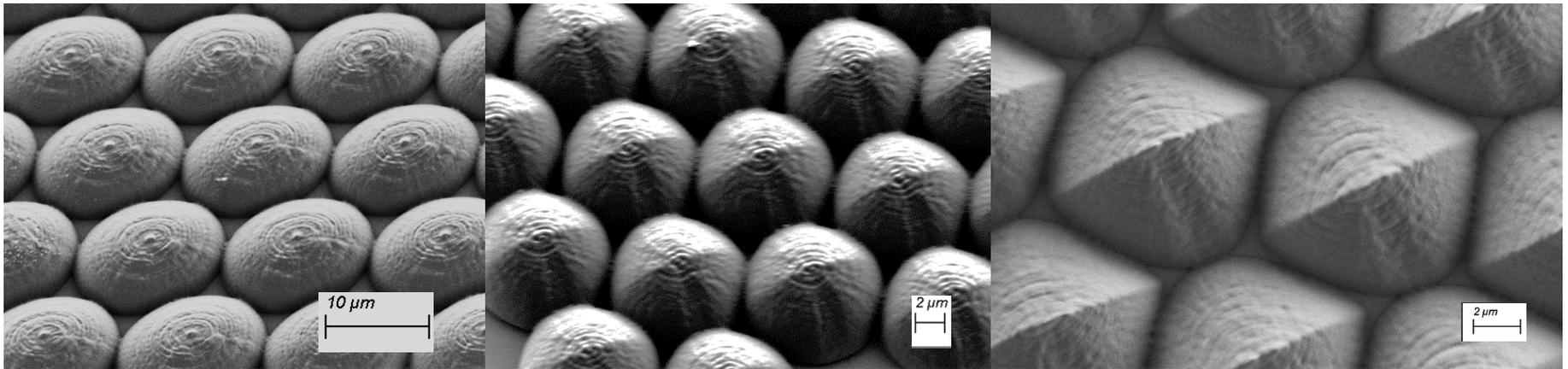
Fig. 11: SEM images of structures printed using 2PP. Left: hemispheres. Middle: structures with  $e = 1$  and  $N = 1.5$ . Right: structures with  $e = 1$  and  $N = 1$ .
