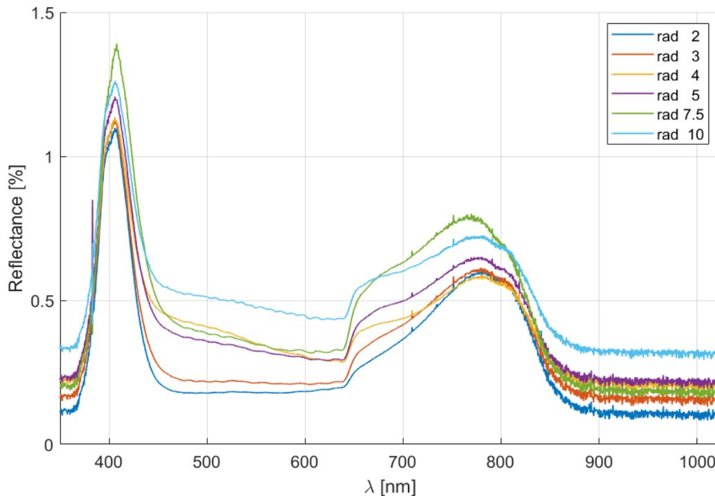
Fig. 13: Reflectance spectra of the printed hemisphere arrays for different radii ( $R_0$ ) in  $\mu\text{m}$ .
