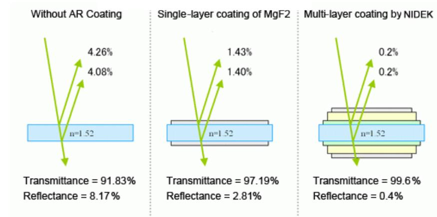
Fig. 1: Example on the effect of SL (middle) and ML (right) AR coating as compared to no coating (left)<sup>3</sup>
