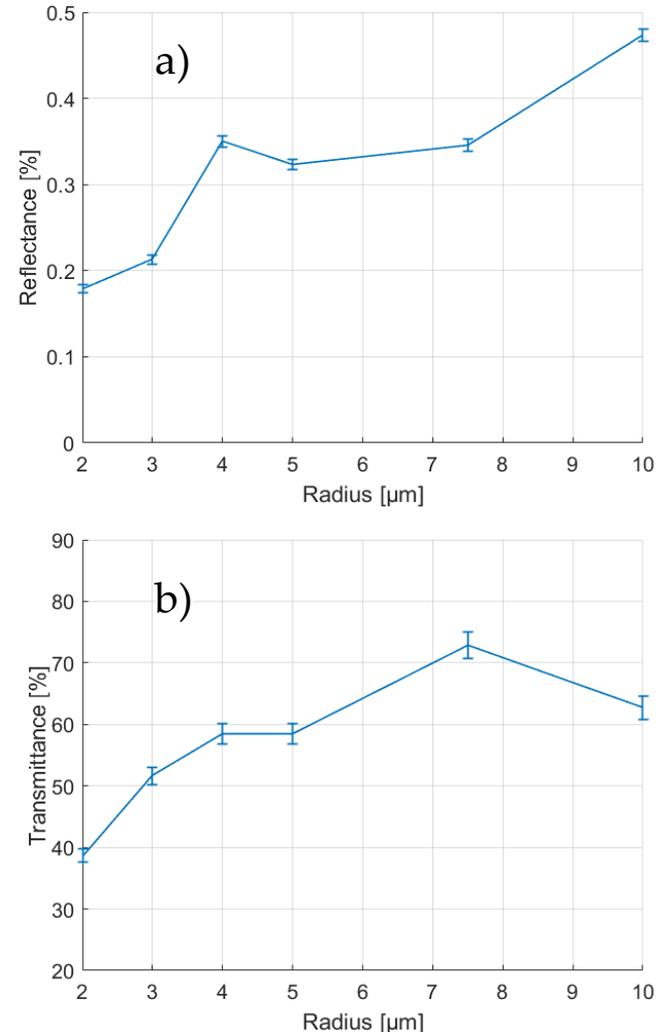
Fig. 14: a) Reflectance at  $\lambda = 550.02$  nm, b) Transmittance measured from the camera
