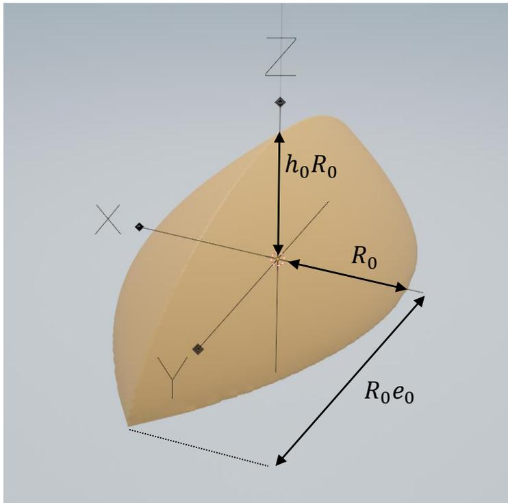
Fig. 9: Example of microlens structures generated with parameters  $R_0 = 5$  arb. unit,  $h_0 = 2$ ,  $e_0 = 2$  and  $N = 1$
