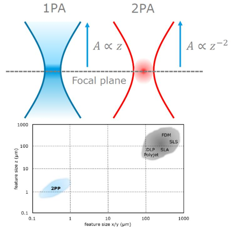
Fig. 10: Principle of two-photon absorption for two-photon printing (2PP)<sup>13</sup>.
