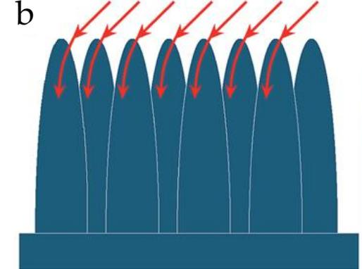
Fig 3: Macroscopic and microscopic rough surface effect on reflectance.<sup>5</sup>
