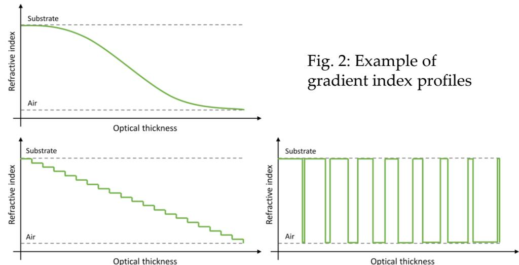
Fig. 2: Example of gradient index profiles
