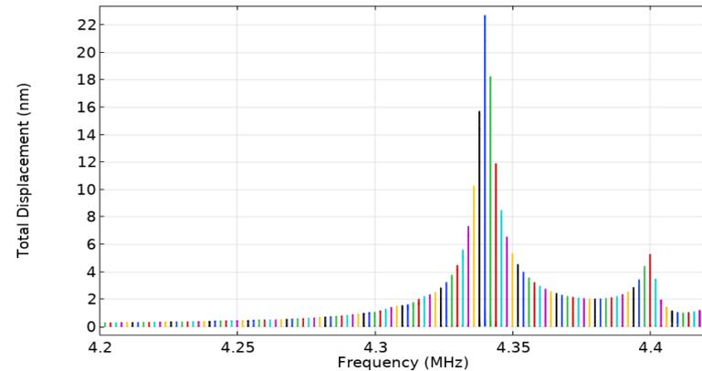
Fig.11. Resonant frequency of QCM for 200  $\mu\text{g}$  added mass.
