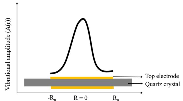
Fig.4. Energy trapping effect of QCM
