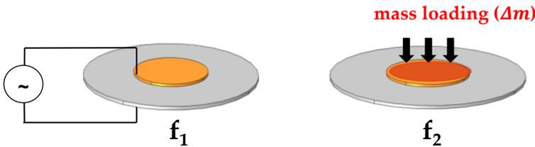
The size of the mass loading area (A) influences mass loading on the QCM, thus affecting the frequency shift ( $\Delta f$ ) and the device sensing performance.
