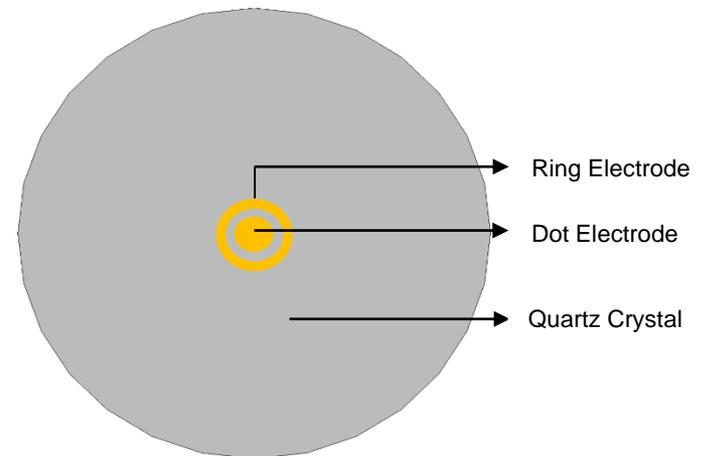
Fig.15. Ring-Dot electrode configuration
