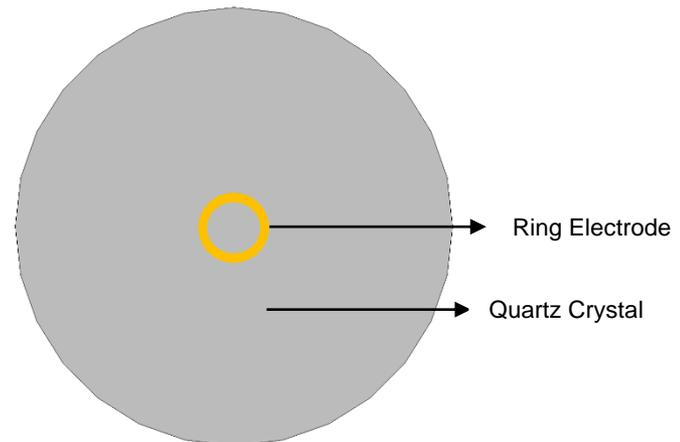
Fig.13. Ring electrode configuration
