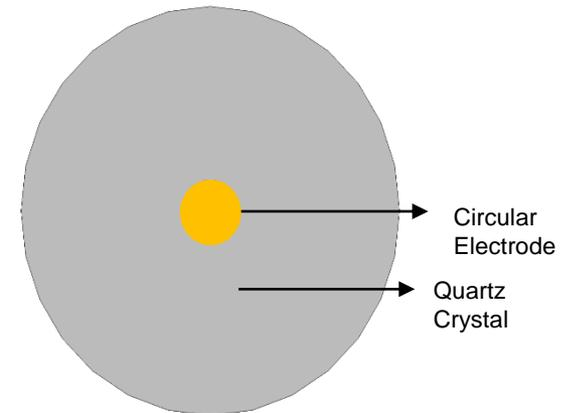
Fig.8. Conventional circular electrode configuration
