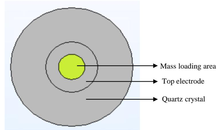
Fig.12. QCM top electrode mass loading area
