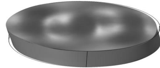
Fig.3. Thickness-shear deformation of a quartz crystal
