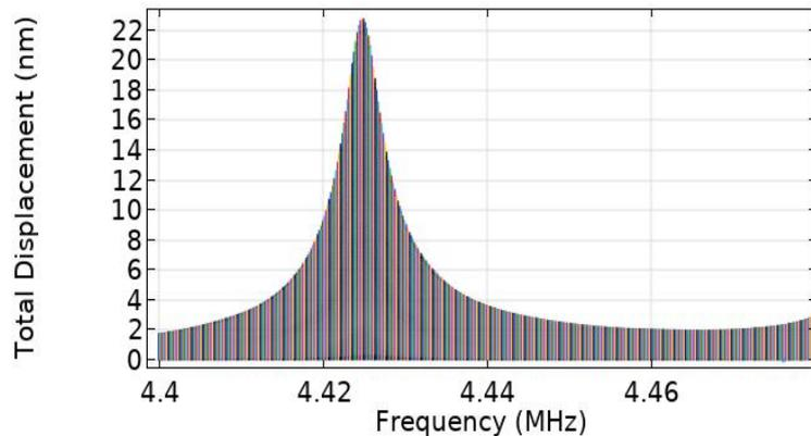
Fig.10. Resonant frequency of QCM for 0 added mass.
