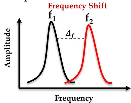
Mass loading on a QCM causes a shift in the resonant frequency. Thus, the sensing performance can be determined by frequency shift using the relation:
