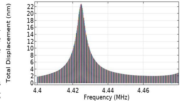
Fig.6. Line plot of Resonant Frequency of QCM
