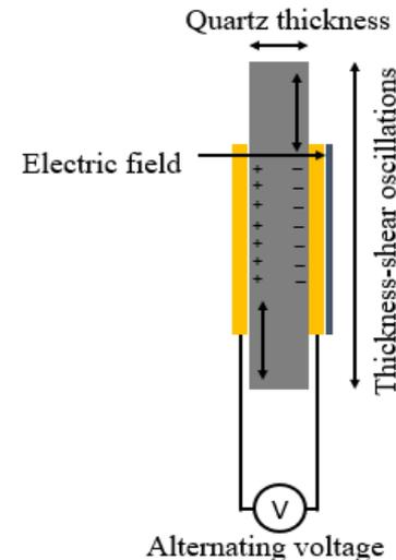
Fig. 2. Quartz Crystal Microbalance operating principle
