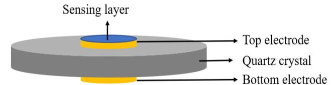
Fig. 1. Quartz Crystal Microbalance Structure (not to scale)
