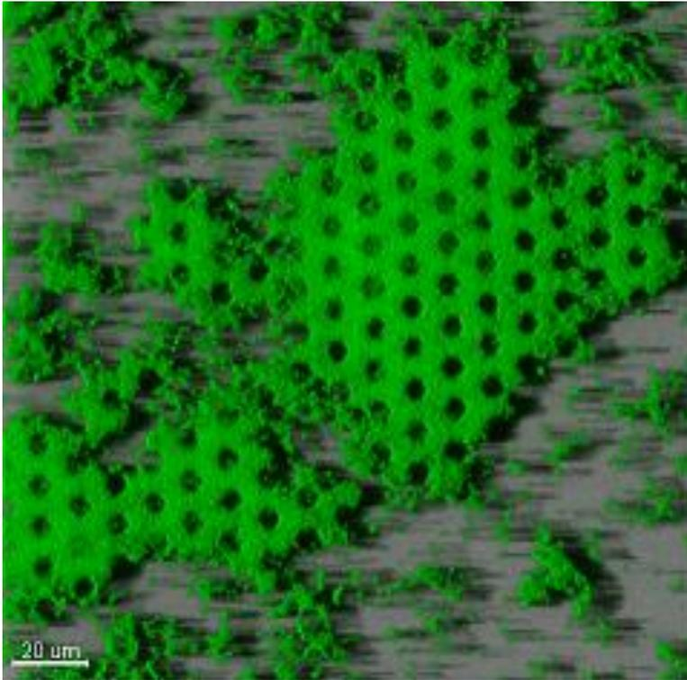
Biofilm grown on honeycomb pillars with side length  $\sim 2.5$   $\mu$ m, width (trench)  $\sim 10$   $\mu$ m and depth  $\sim 12$   $\mu$ m. (biofilm incubation with low stirring after 48 hours in 25  $^{\circ}$ C)
