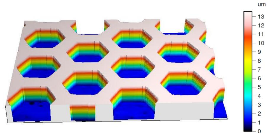
3-D profile of honeycomb pits with taken by optical profiler (Sensofar PLu Neox 3D) side length  $a \sim 5 \mu\text{m}$  and width  $d \sim 2.5 \mu\text{m}$  and depth  $\sim 12 \mu\text{m}$ . The color code represents heights from blue (low) to white (high).
