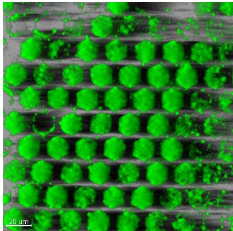
Biofilm grown on honeycomb pits with side length  $\sim 10$   $\mu$ m, width (trench)  $\sim 5$   $\mu$ m and depth  $\sim 12$   $\mu$ m. (biofilm incubation with low stirring after 48 hours in 25  $^{\circ}$ C)
