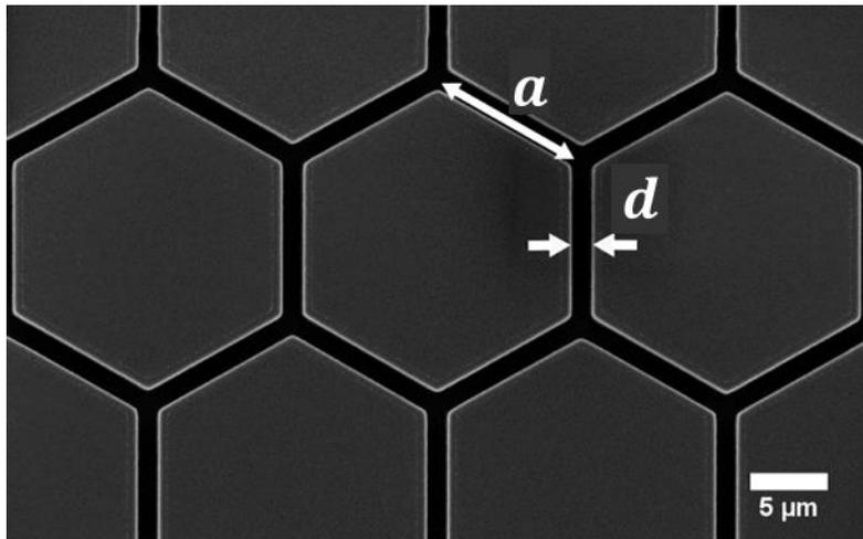
Silicon patterned microstructure of an array of honeycomb pillars with side length  $a \sim 10 \mu\text{m}$  and trench width  $d \sim 1 \mu\text{m}$ .
