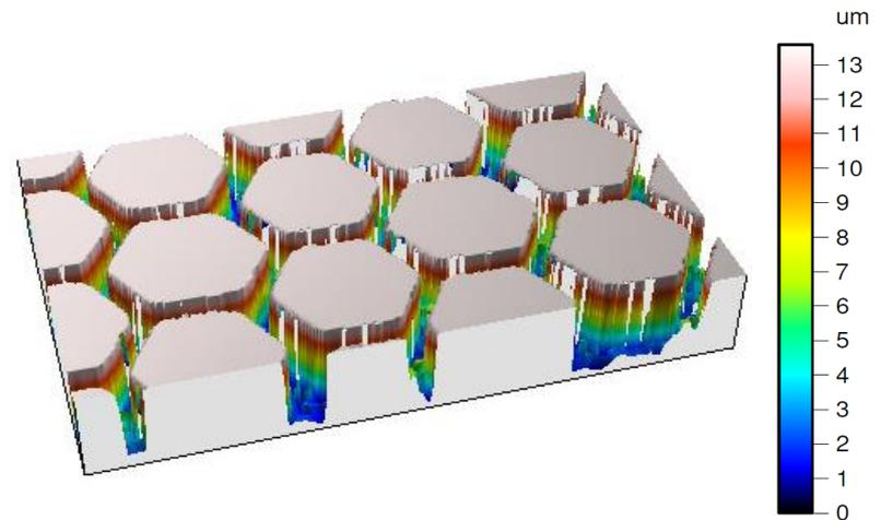
3-D profile taken with optical profiler (Sensofar PLu Neox 3D)  $d \sim 1 \mu\text{m}$ ,  $a \sim 10 \mu\text{m}$  and height  $\sim 13 \mu\text{m}$ . The color code represents heights from blue (low) to white (high).
