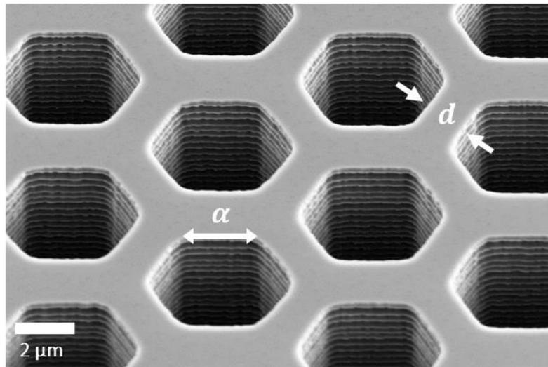
Silicon patterned microstructure of an array of honeycomb pits with side length  $\alpha \sim 5 \mu\text{m}$  and trench width  $d \sim 2.5 \mu\text{m}$ .
