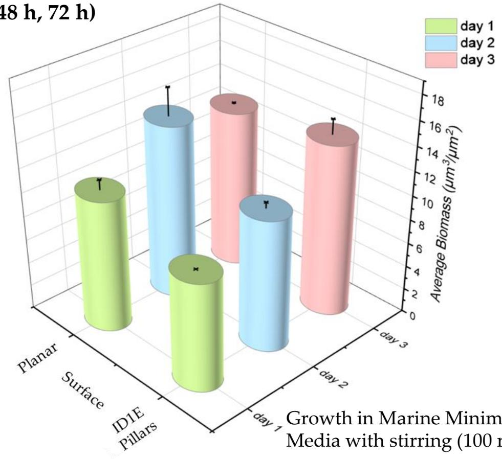
Growth in Marine Minimal Media with stirring (100 rpm)
