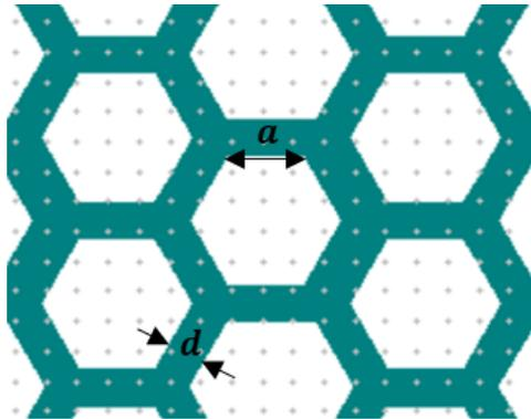
RID1E pits with side length  $a \sim 5 \mu\text{m}$  and width  $d \sim 2.5 \mu\text{m}$
