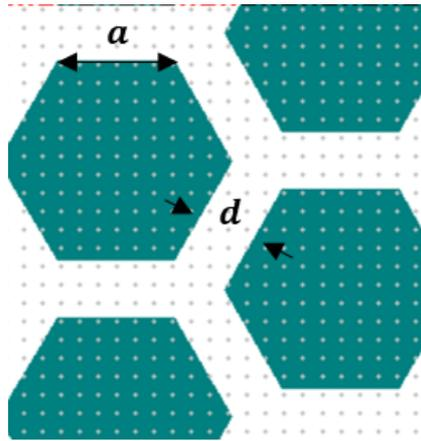
ID1E: Honeycomb pillars with side length  $a \sim 5 \mu\text{m}$  and width  $d \sim 2.5 \mu\text{m}$
