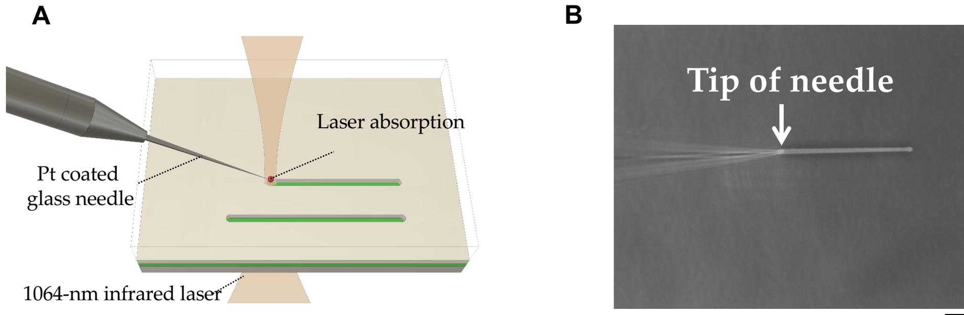
**Fig.3.** Detailed drawings of agarose microfabrication with Pt-coated microneedle (A) Schematic figure. (B) Phase contrast image of agarose microfabrication. Bar, 10  $\mu\text{m}$ .
