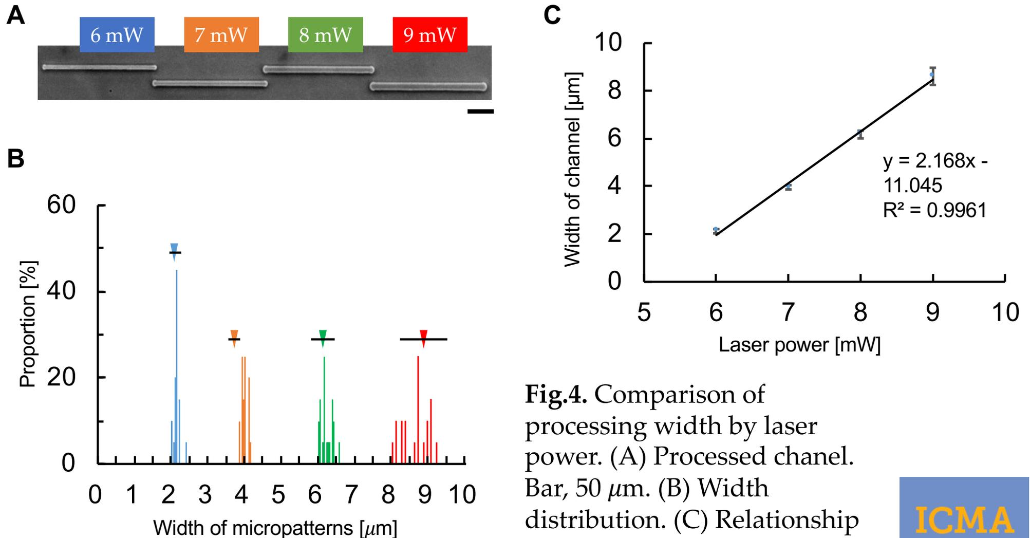
**Fig.4.** Comparison of processing width by laser power. (A) Processed channel. Bar, 50  $\mu\text{m}$ . (B) Width distribution. (C) Relationship between laser power and width.
