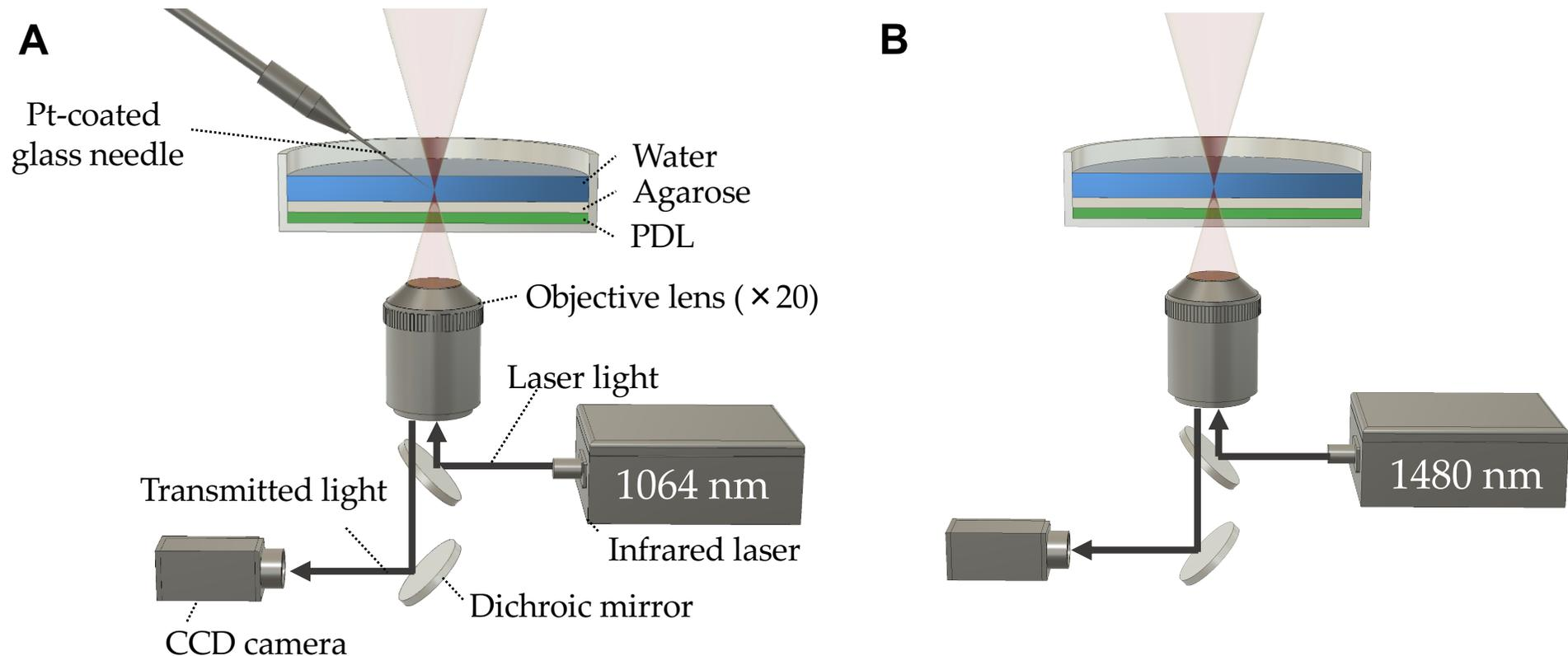
**Fig.2.** Two ways of system design: (A) Microneedle absorbance technology, (B) direct absorbance technology.
