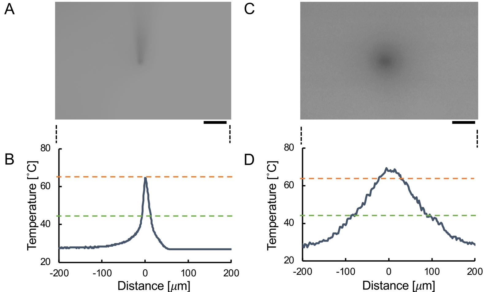
**Fig.6.** Comparison of the heating ranges of agarose microfabrication technologies. (A)(B) Microneedle method. (C)(D) Direct absorbance method. Bars, 50  $\mu\text{m}$ .
