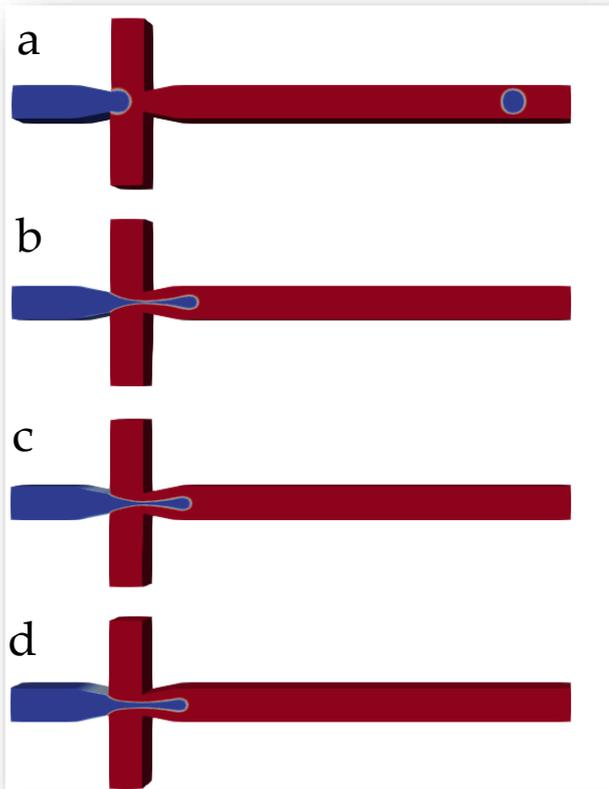
Fig 5 – Effect of increasing the polymer concentration on droplet formation
