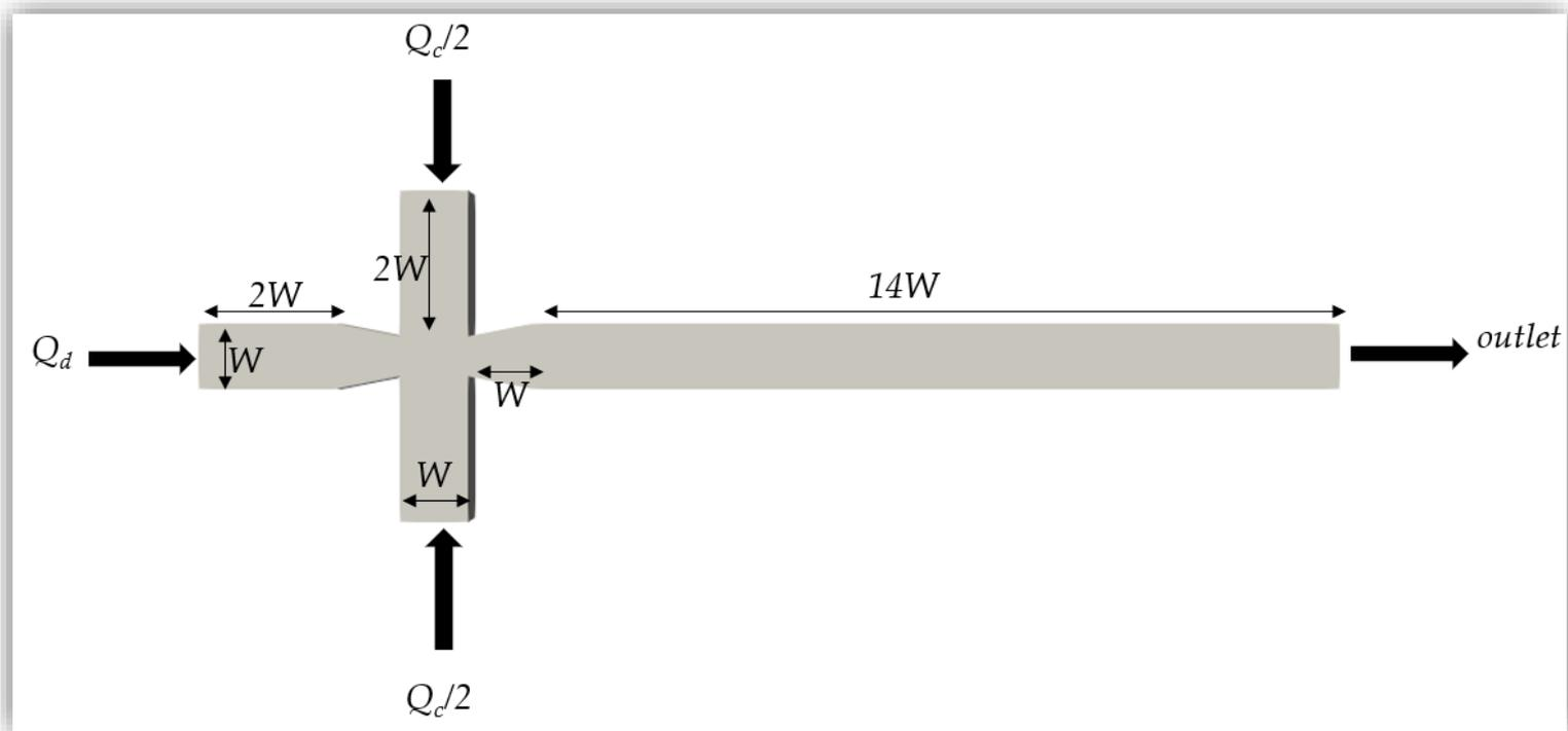
Fig 2 - Geometry of studied cross-junction
