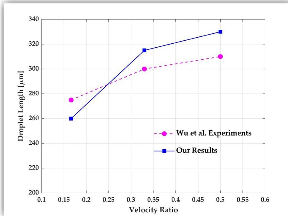
Figure 4 - Droplet length results compared against the experimental results of Wu et al. [6] for  $U_o = 0.00252$  (m/s),  $\sigma = 30$  (mN/m), and  $\mu_o / \mu_w = 0.416$
