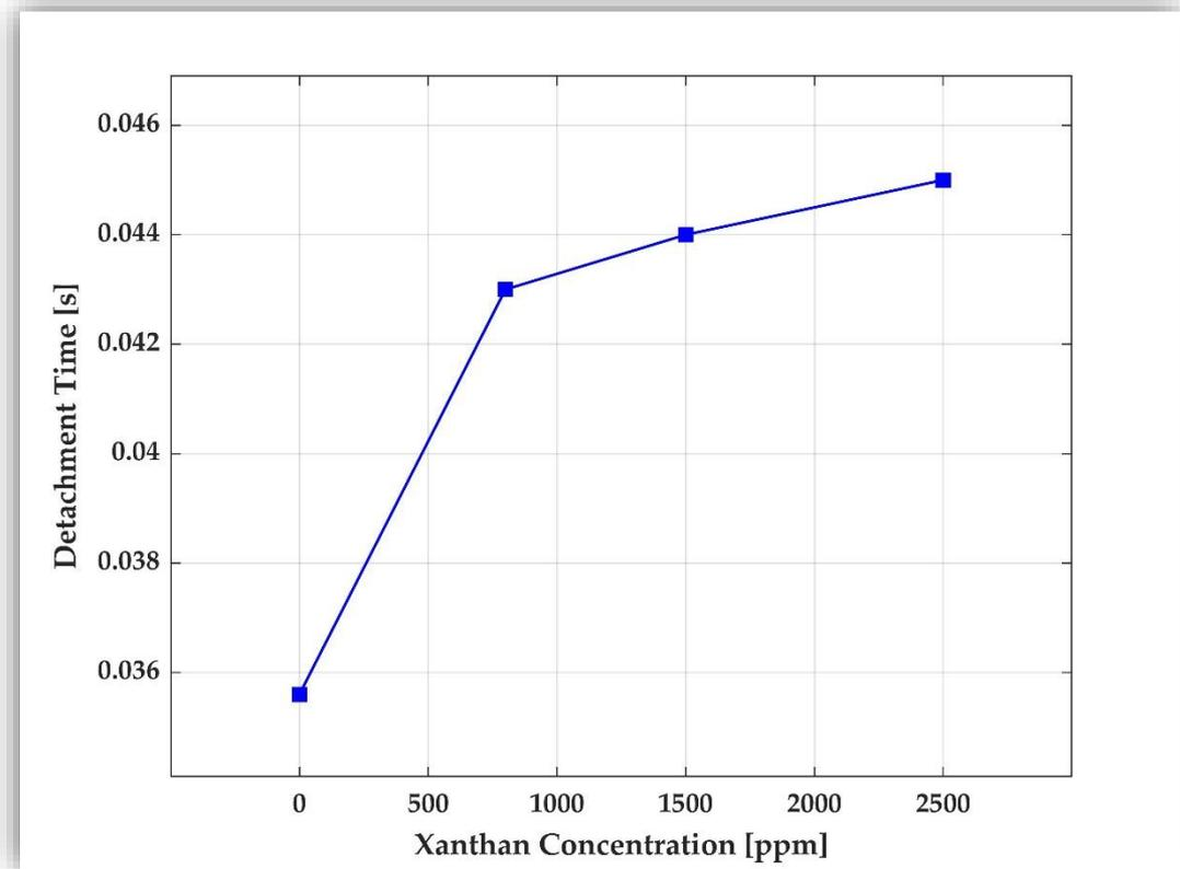
Fig 6 – Effect of the polymer concentration on droplet detachment time
