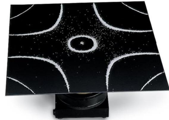
**Fig. 3. Chladni plate with the sand on top forming a Chladni Figure [4]**
