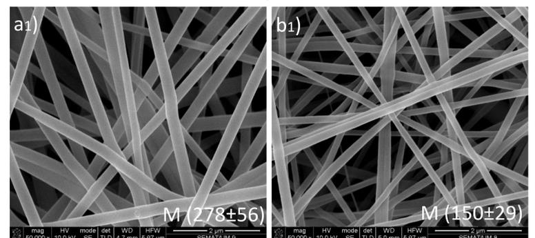
Figure 1: FEG-SEM image of 80/20 uncrosslinked (a) PVA/CA and b) PVA/CNC and crosslinked (a1) PVA/CA and b1) PVA/CNC nanofibers (n=50) with respective means (M) of nanofibers diameters.
