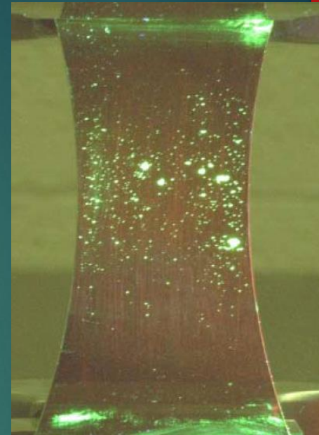
AA7050 specimen; fatigued then loaded to reveal cracks (dye penetrate)
